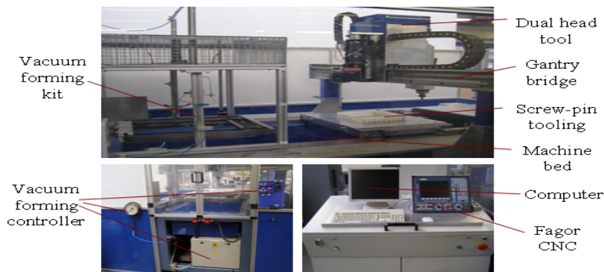
Fig.5 The completed HAVES
